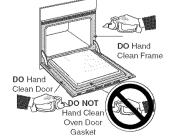
Use soap & water to thoroughly clean the top, sides and front of the oven door. Rinse well. You may use a glass cleaner on the outside glass of the oven door. **DO NOT** immerse the door in water. **DO NOT spray or allow water or the glass cleaner to enter the door vents.** DO NOT use oven cleaners, cleaning powders or any harsh abrasive cleaning materials on the outside of the oven door.
